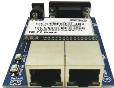
HLK-RM04 Uart WIFI with internal Antenna
