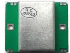
Microwave Sensor Module HB100
