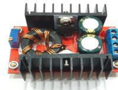
DC-DC BOOST CONVERTOR Step UP I/P:- 10V- 32V O/P:- 12V TO 35V / 6A
