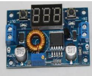
XL4015 LED MODULE I/P:- 4V- 38V O/P:- 1.25V-36V / 5A
