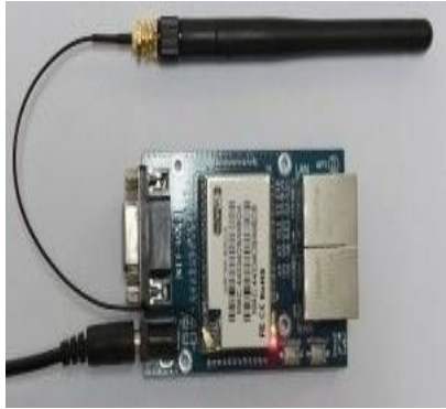
HLK-RM04 Uart WIFI with External Antenna
