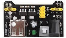
USB Power Module 3.3V 5V
